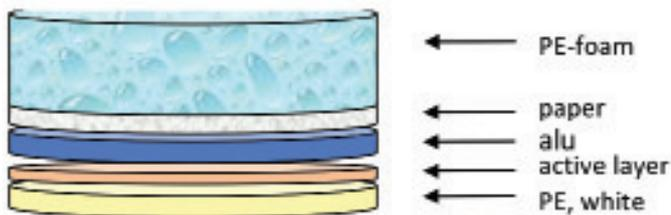
Figure 1: Design of the ALKOvin™ active liner adsorbing VSCs in bottled wines.
